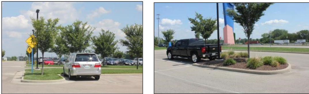
Figure 1123-B: The above images show different options for landscaped islands with the top image illustrating landscaped islands that run the full length of parking spaces. The bottom image illustrates a smaller landscaped island at the end of a parking bay.
