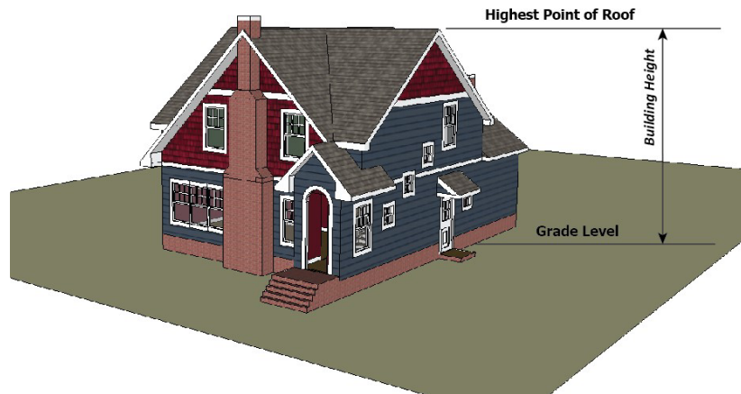
Figure 1115-H: Measurement of building or structure height
