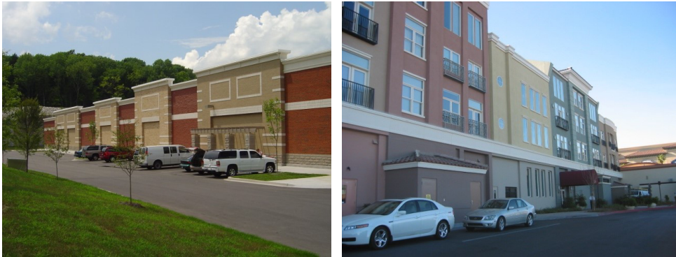
Figure 1119-D: This figure shows two methods of using architectural features to create wall surface relief on wall elevations that are not the primary elevation.
