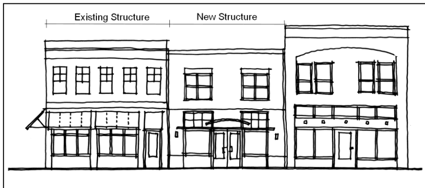
Figure 1119-E: This image illustrates how existing and new structures divide the entire façade plane into smaller components through the use of pilasters, storefronts, height variation, and material variations.
