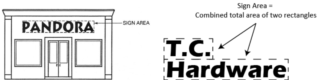
Figure 1127-C: Illustration of sign area calculation for two differently shaped wall signs with individual letters.
