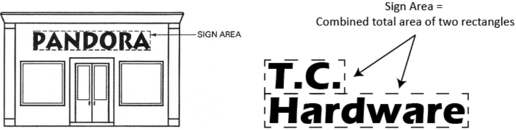
Figure 1127-C: Illustration of sign area calculation for two differently shaped wall signs with individual letters.
