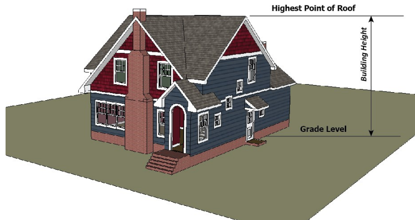
Figure 1115-H: Measurement of building or structure height
