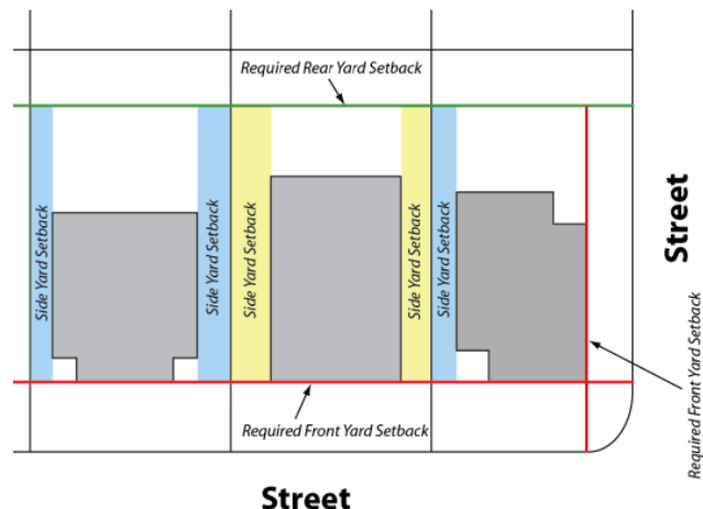
Figure 1115-A: Measurement of typical front, side, and rear yard setbacks.
