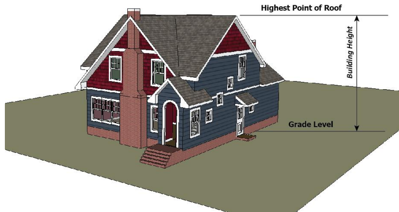
Figure 1115-H: Measurement of building or structure height
