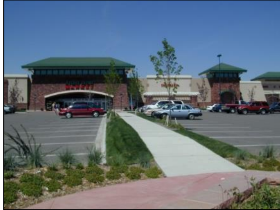
Figure 1125-D: This photograph illustrates how a sidewalk connecting the public sidewalk to the business can be integrated into the required landscaping.
