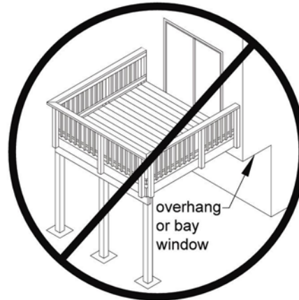
Figure 18: No Attachment to House Overhang
